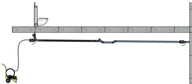
Figure 2. Illustration of removal of soft scaling using a portable sewer jetter.
