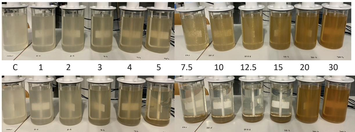
Figure 6.1 Jar Test for influent greywater using PIX-111 during slow mixing (upper) and after settling for 30 minutes (lower). Molar ratios listed in between the two timepoints.
