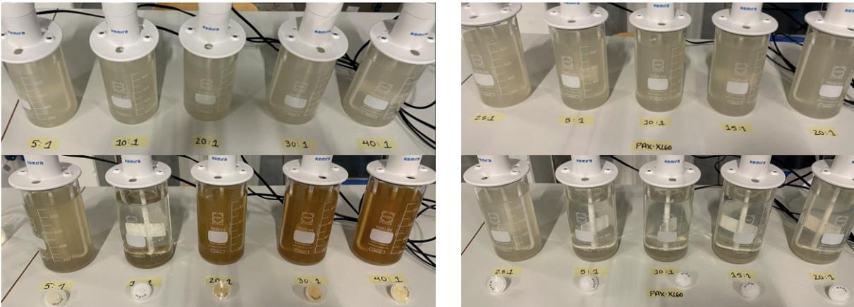
Figure 5.3 Jar tests on influent greywater using PIX-111(left) and PAX-XL60 (right) during the proof of concept stage.
