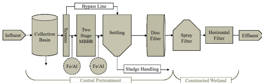
Figure 3.2 Treatment scheme at the proposed Östra Ramlösa plant. Proposed chemical precipitation points denoted with dotted lines (simplified, coagulation and flocculation tank placement decided upon final precipitation placement decision).
