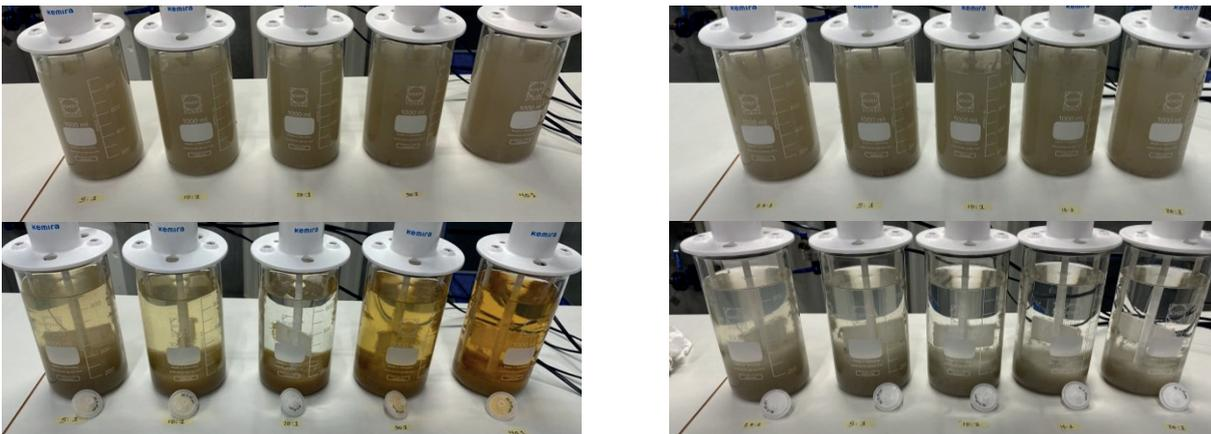
Figure 5.4 Jar tests on biologically treated water using PIX-111(left) and PAX-XL60 (right) during the proof of concept stage.
