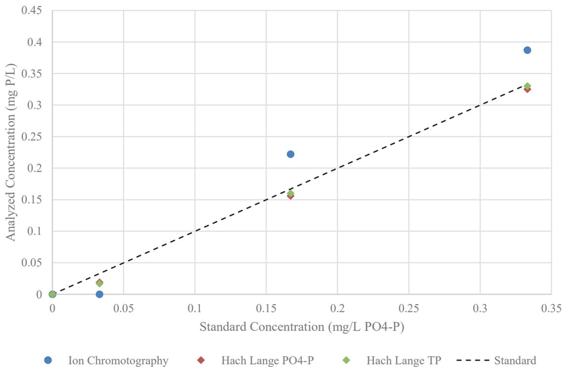
Figure 5.5 Comparison of analytical methods for phosphorous detection.
