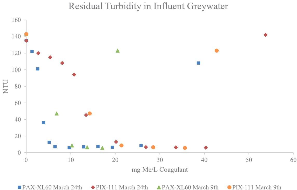
Figure 6.5 Residual Turbidity after Coagulation in Influent Greywater
