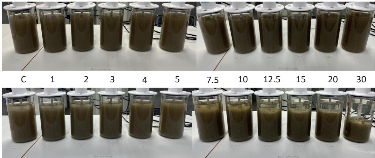
Figure 6.6 Jar Test for biologically treated greywater using PIX-111 during slow mixing (upper) and after settling for 30 minutes (lower). Molar ratios listed in between the two timepoints.
