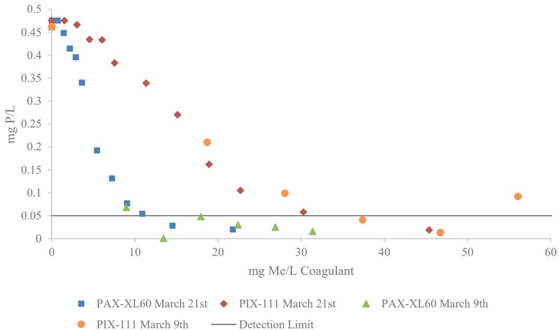
Figure 6.8 Residual Total Phosphorous Concentration after Coagulation in Biologically Treated Greywater. The line at 0,05 mg P/L indicates the detection limit of the Hach Lange cuvettes used. All values below the line are considered undetectable even though a numerical reading was obtained
