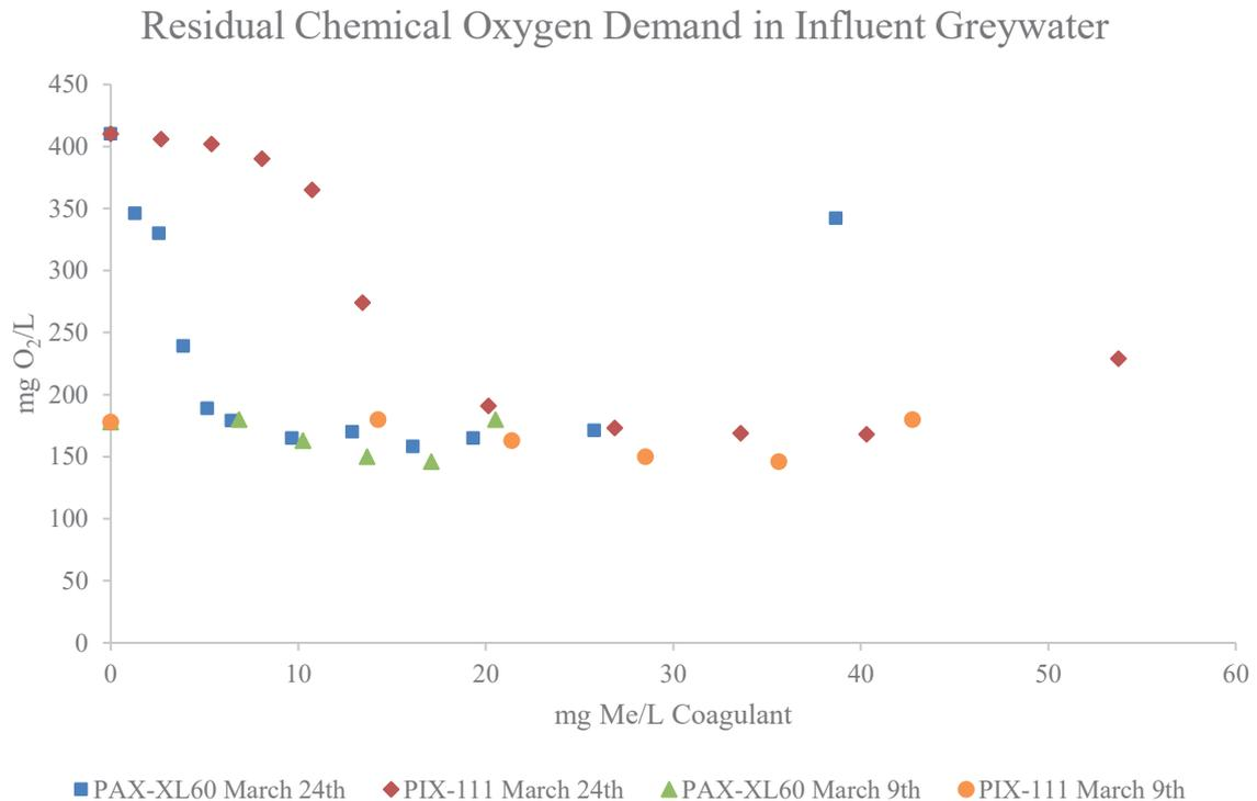
Figure 6.4 Residual Chemical Oxygen Demand after Coagulation in Influent Greywater
