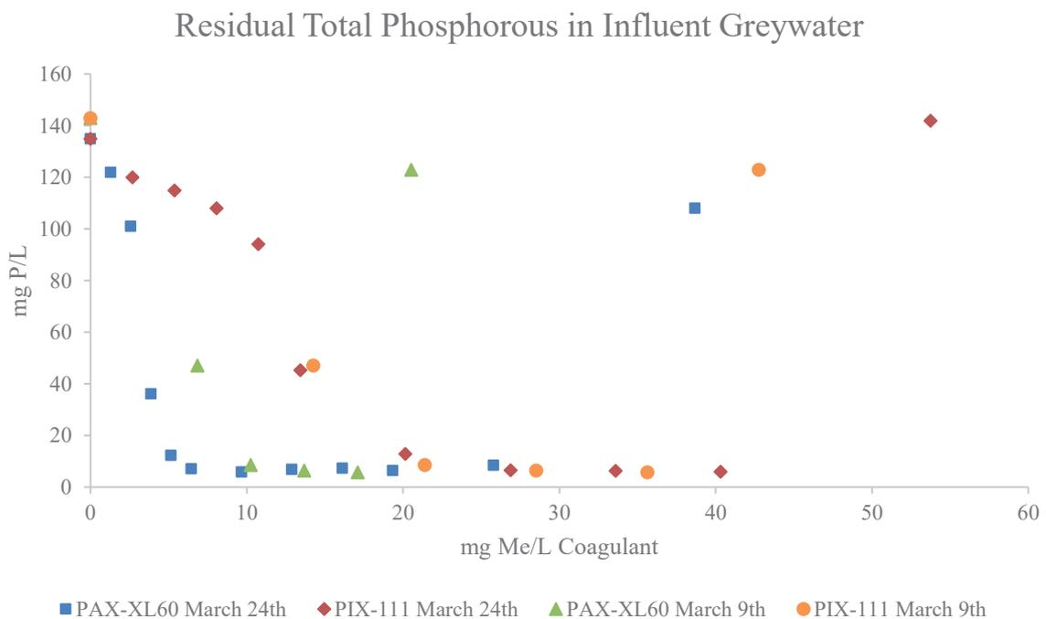
Figure 6.3 Residual Total Phosphorous after Coagulation in Influent Greywater
