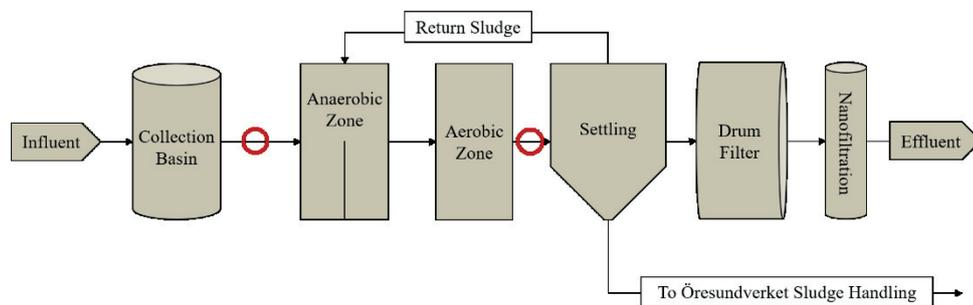
Figure 3.1 Treatment scheme for greywater at RecoLab pilot plant for Oceanhamnen during the spring of 2022. Sampling points circled in red.
