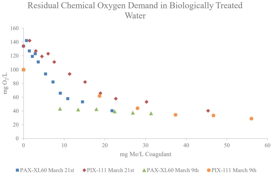
Figure 6.9 Residual Chemical Oxygen Demand after Coagulation in Biologically Treated Greywater.
