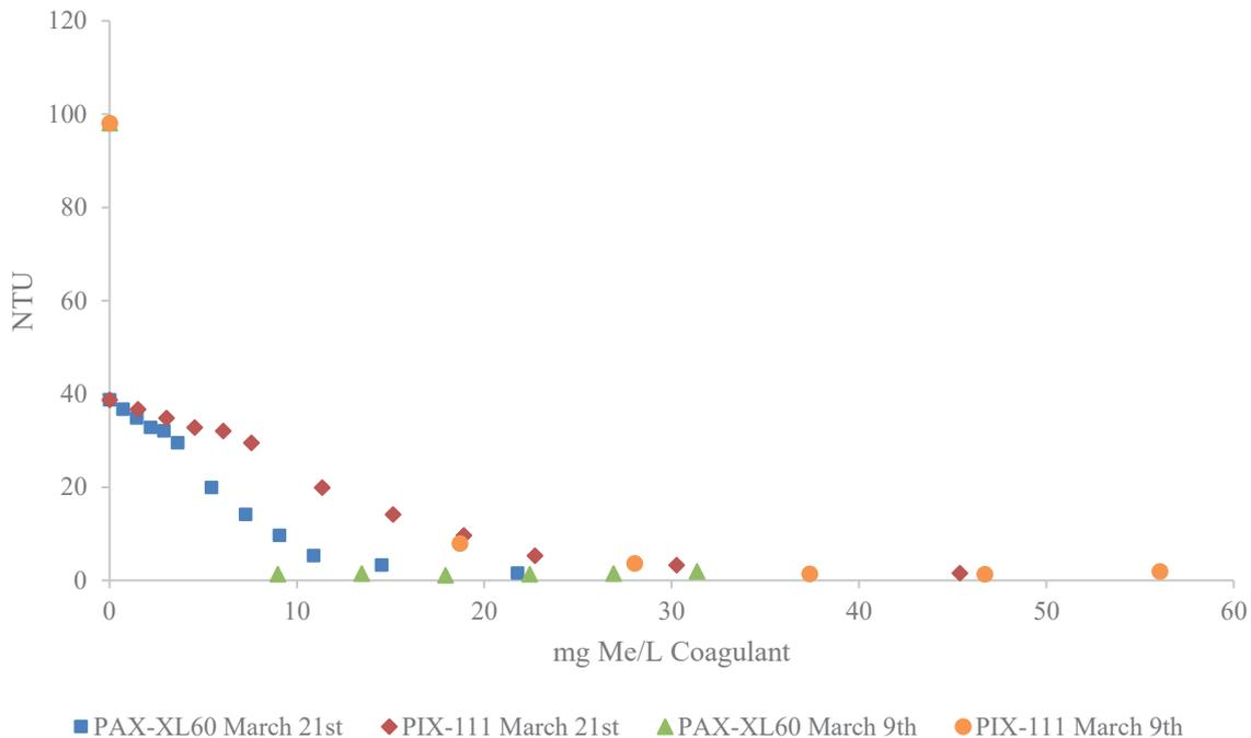
Figure 6.10 Residual Turbidity after Coagulation in Biologically Treated Greywater.
