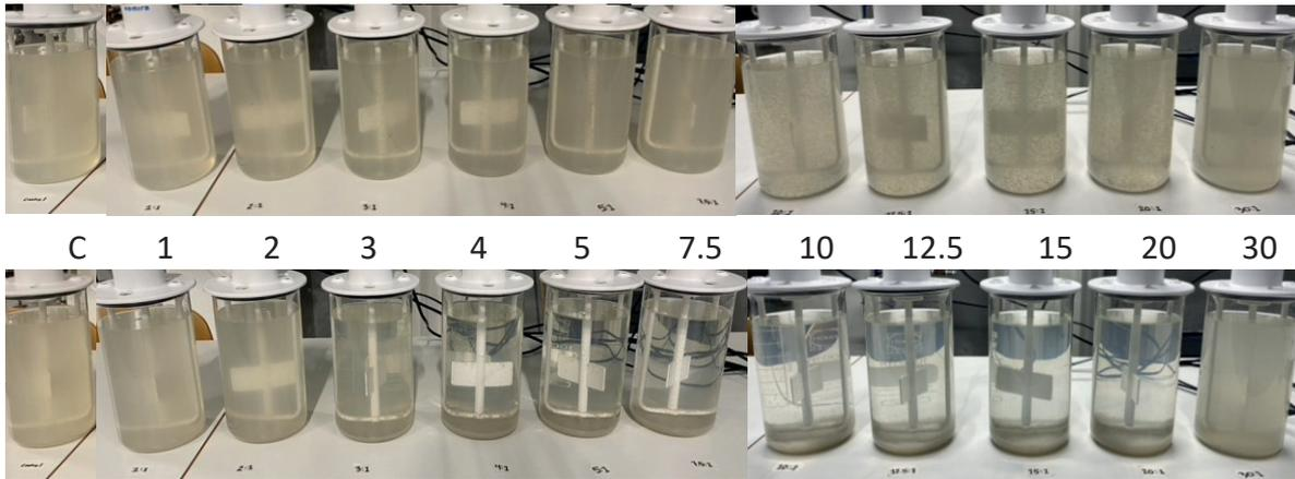
Figure 6.2 Jar Test for influent greywater using PAX-XL60 during slow mixing (upper) and after settling for 30 minutes (lower). Molar ratios listed in between the two timepoints.
