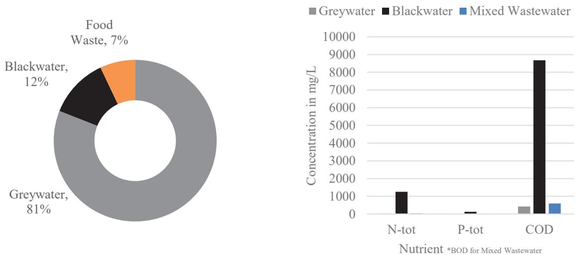
Figure 2.1 Wastewater flow percentages (left) and nutrient concentrations (right) in water entering RecoLab and Öresundsverket in Helsingborg, Sweden.
