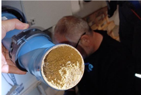
Figure 4.1 Severe deposit formation in the bend right before pipe leaves the building
